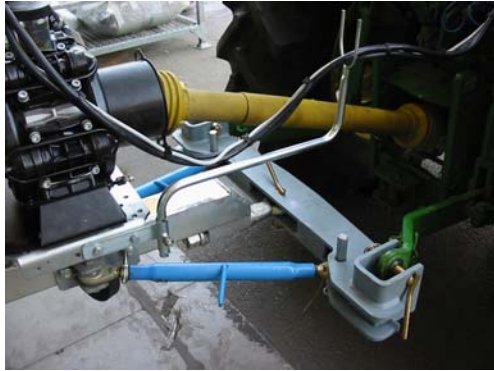
Tractor coupling for homologated Towed machines in work position (not suitable for road use).
